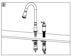
Make sure the O-ring is placed at the bottom of the spout and valve body, then install the spout and valve body through the hole in the sink, and the valve body is installed on the right side of the spout.
