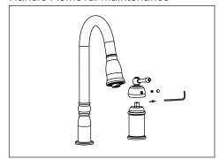
Turn off water and relieve pressure! Detach handle button using a small flathead screwdriver, unscrew set screw using Allen Wrench and take off handle.
