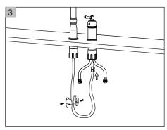
Connect the pull-down hose to the shorter hose at the bottom of the valve body and tighten it. Install the weight on the lower end of the vertical part of the pull-down hose and tighten it with a cross screw driver until the weight does not move.
