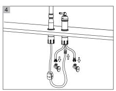
Connect the hot and cold water supply lines to the corresponding hot and cold water supply valves and tighten them with a wrench.
