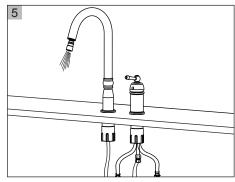
After installation is complete, remove spray head and rotate handle to the close position, turn water supply valves on, and check all connections for leak, then open the hot and cold water supply valve and tap control valve completely for one minute to flush the residue in the pipe.
