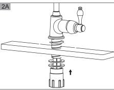
Install without Deck Plate. Make sure the O-RING is placed onto the bottom of Base Ring. Install faucet through hole in sink. From underside sink, attach mounting assembly Position faucet on sink properly and tighten Mounting Nut.
